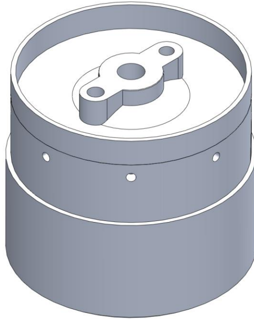
Figure 8. Forward Bulkhead (isometric view)
