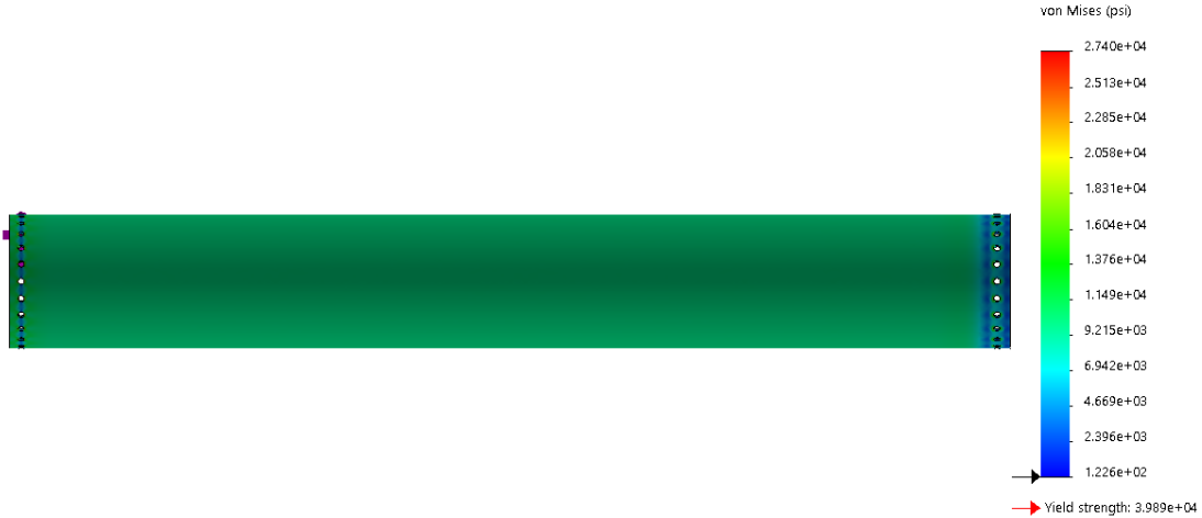
Figure 92. Combustion Chamber Global Stress Distribution
