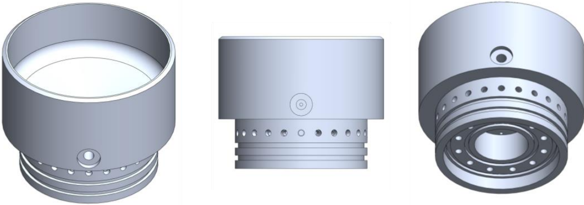
Figure 13: Injection Bulkhead (three views)
