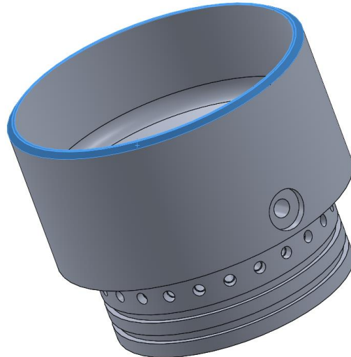
Figure 74. Injection Bulkhead Fixed Geometry
