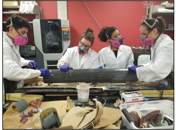
Composites team post-processing Noctua III airframe
