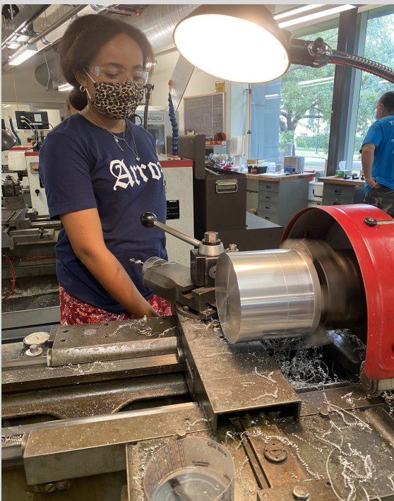
Machining Oxidizer Tank Bulkhead
